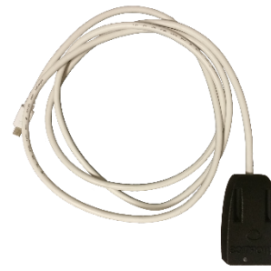
Figure 3c (2015): Single custom displayport connection, able to support single and dual display devices using a single cable. Used for current generation Cinoptics devices. Uses a fixed end-of-cable cablecombiner to transfer power and USB over a Displayport connection.
