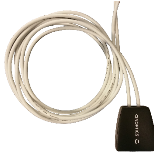
Figure 3b (2013): Double custom displayport connection, used for current generation dual display Cinoptics devices. It uses a fixed end-of-cable cablecombiner to transfer power and USB over a Displayport connection. Requires separate video signals for left and right displays.
