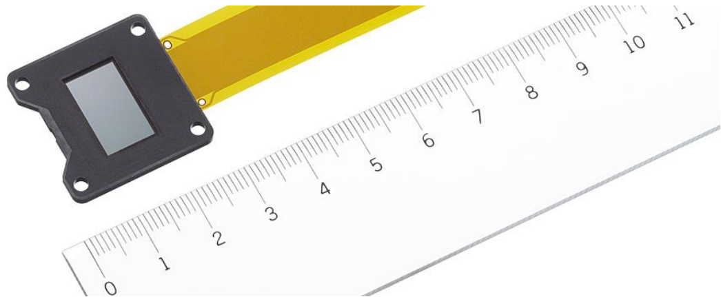
Figure 2: OLED Microdisplay as used in Cinoptics AIRO II
